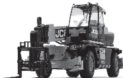
Rotating Forklift - Max Lift height 83' - Max reach 70'2" - Lift Capacity 12,125 lbs
