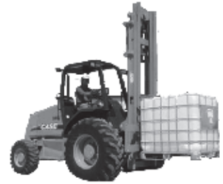
6000 lb. Fork Lift - 21' Lift - Straight Mast
